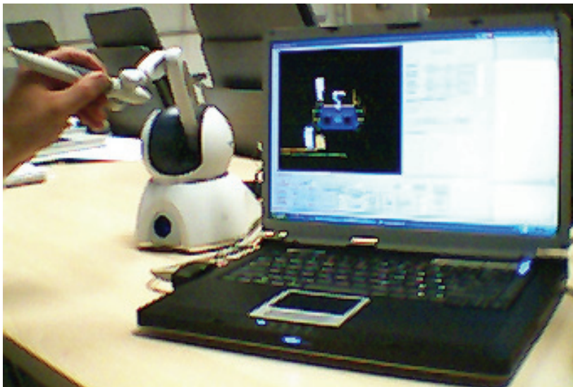
Fig. 6. Off-line programming of the telerobot using a haptic device
