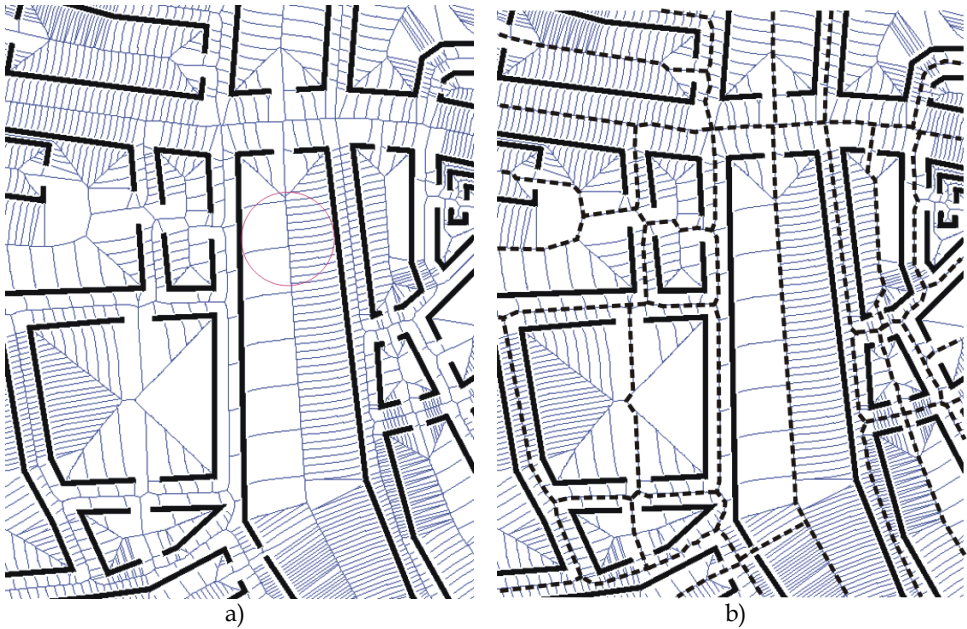
Fig. 4. Construction of the GVD: a) ordinary Voronoi diagram (light lines), b) GVD (dotted lines)
