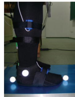
Fig. 14. Acquiring and measuring system, Biopac type, for the foot and lower leg linear accelerations
