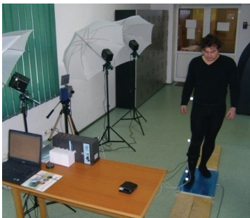
Fig. 14. Acquiring and measuring system, Biopac type, for the foot and lower leg linear accelerations
